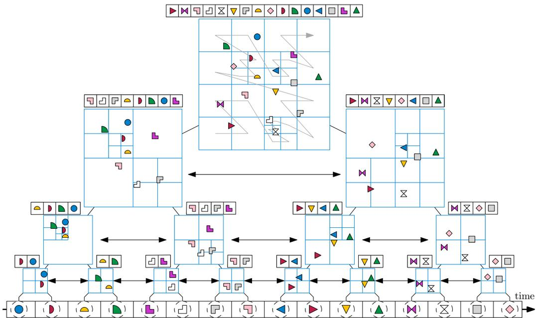
Figure 10: Decomposition tree over temporal points. Each temporal point has a corresponding geometric point with coordinates in  $\mathbf{R}^2$ . Each node stores the quadtree and z-order of the points in its subtree.
