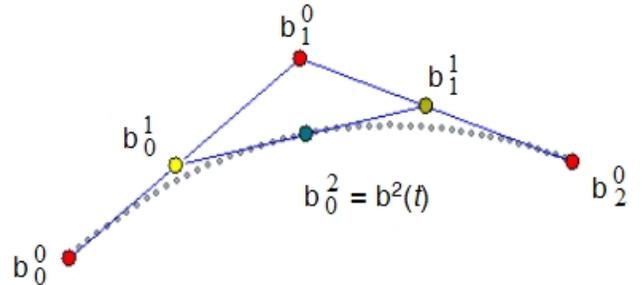
Figure 1: A Quadratic Bézier Curve Traced by an m-Linkage
