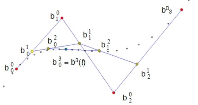
Figure 4: A Cubic Bézier Curve Traced by an m-linkage
